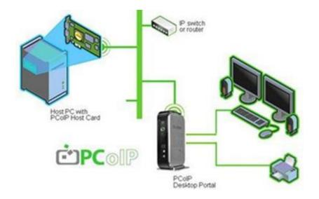
With the Teradici's PCoIP remote acceleration host card, users can achieve 100 percent color matching with lossless imaging over affordable IP networks in tandem with any of the Zero Client workstations. This is achieved through Teradici's innovations focused on pixel-level transmission.
